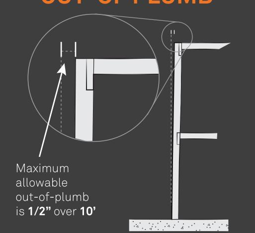
An out-of-plumb upright means that it is not exactly vertical. Always look in the cross-aisle and down-aisle directions.
