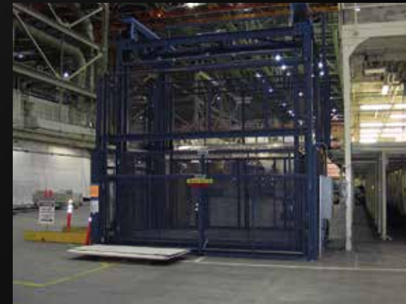
Aeronautics Lift – M Series Mechanical VRC Moves materials to assist with the production of airplanes. 5,000 lbs. lifting capacity; 18' 7" lift travel; 3 levels of service; 27' per minute travel speed.
