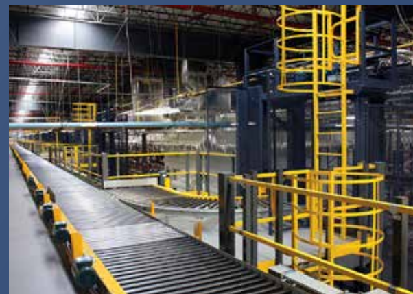
Home Appliance Lifts – M Series Mechanical VRC Ten lifts installed as a mezzanine application, including a conveyORIZED system. 1,200 lbs. lifting capacity; 200' per minute travel speed.
