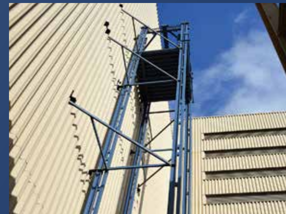
Waste Incinerator Lift – F Series Mechanical VRC Lift moves contraband materials seized by law enforcement authorities from the ground level to an elevated incinerator. 15,000 lbs. lifting capacity; 79' lift travel; 37' per minute travel speed.
