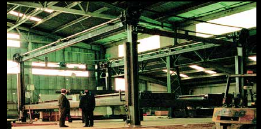
Fuel Cell Energy Material Lifts – F Series Mechanical VRC Combination of two material lifts. The first is a screw lift mechanism. The second is a material lift that traverses sideways and lowers onto the first lift. 5,000 lbs. lifting capacity; 18' lift travel; 3 levels of service; 17' per minute travel speed.
